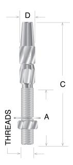
Electroline synthetic rope fittings for Kevlar rope with braided jackets excel in meeting the need for a quick, reliable end termination. These fittings use a swagless design with an internal taper pin that allows them to be installed in the field without special tools or complicated processes. They are selected for both the rope size and rated rope strength. This fitting features a threaded stud that can be used to connect and tension the rope to a fixed point.
