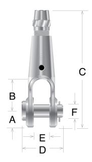
Electroline's industrial series clevis (fork/jaw) socket fitting includes a pin and cotter pin. It features a swageless rope termination that can be quickly installed in the field without special tools or processes.
