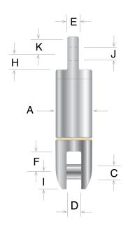
Electroline's Model SSP-65 industrial swivel is designed for sub-surface (below water) marine applications. It features an eye-end fitting and a clevis (fork/jaw) fitting. Constructed from stainless steel, the oil-filled housing is sealed and pressure compensated to prevent water entry.
