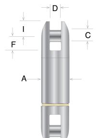
Electroline's Model SSP-67 industrial swivel is designed for sub-surface marine applications and features two clevis (fork/jaw) fittings with included pins. Constructed from stainless steel, the oil-filled housing is sealed and pressure compensated to prevent water entry.
