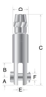
Electroline synthetic rope fittings for Kernmantle rope are supplied with the SAR1000 series internal plug. The sleeve has no exposed thread when assembled and is retained in the socket with a set screw. This fitting features a clevis (fork/jaw) with an included pin. The swagless termination allows it to be installed in the field without special tools or processes.
