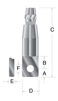
Electroline synthetic rope fittings for Kernmantle rope are supplied with the SAR1000 series internal plug. The sleeve has no exposed thread when assembled and is retained in the socket with a set screw. This fitting features an eye fitting and a swagless termination, allowing it to be installed in the field without special tools or processes.
