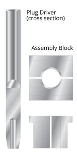
Electroline's swagless rope terminations can be quickly installed in the field without the need for expensive tools, chemicals, pressure, or heat. Using an assembly kit can speed up the installation process. The assembly block helps prevent damage to the rope and the plug driver can help seat the plug as well as assist with flaring the rope strands. Electroline's assembly instructions demonstrate how to use the assembly kit when terminating a rope.
