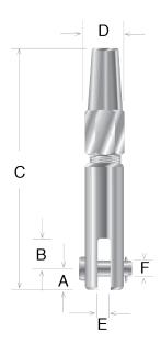
Electroline synthetic rope fittings for Kevlar rope with braided jackets excel in meeting the need for a quick, reliable end termination. These fittings use a swagless design with an internal taper pin that allows them to be installed in the field without special tools or complicated processes. They are selected for both the rope size and rated rope strength.
