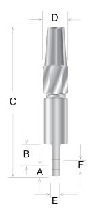
Designed for Kevlar ropes with a braided jacket, this fitting features an eye connector and a swageless termination that allows the fitting to be quickly installed in the field without special tools or processes.
