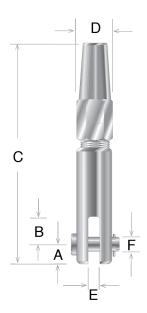
Electroline synthetic rope fittings for Kevlar ropes with extruded jackets excel in meeting the need for a quick, reliable end termination. The fittings perform on polyurethane, Nylon II, and Hytrel jacket materials for ropes with the following construction: standard wire rope, contra-helical, parallel, and electro-mechanical. This fitting features a clevis (fork/jaw) connection and a swageless rope termination, allowing it to be quickly installed in the field without special tools.
