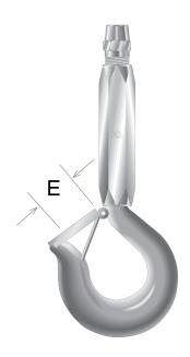
Optional safety latch for Electroline's swiveling and non-swiveling hooks. Select the option that matches the size of the rope being used with the hook fitting. Modification to the hook may be required for installation.
