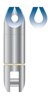
Attaching a wire or synthetic rope to a swivel can be accomplished with a swivel that contains the Electroline® fitting on one side of the swivel. If thimbles with clips are desired, solid core thimbles are recommended. The cast-steel thimbles are zinc-plated and are designed to limit rope wear by preventing the rope from extending beyond the diameter of the swivel.
