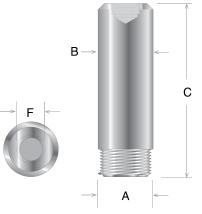
This is a replacement pin for <u>6000 Series Gold Band<sup>m</sup> Swivels</u> with a clevis fitting. To select the correct pin, match the last two digits to the swivel's product ID number with the swivel model number for the pin. *For example, a Model 64 Swivel with product ID 6425 would use the pin for 6x25 swivels.*
