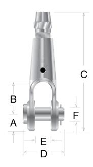
Electroline's industrial series clevis (fork/jaw) socket fitting includes a pin and cotter pin. It features a swageless rope termination that can be quickly installed in the field without special tools or processes.
