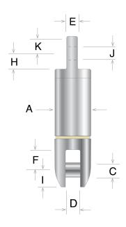
Electroline's Model SS-65 industrial ocean surface swivel is designed for above-water applications and features an eye-end fitting and a clevis (fork/jaw) fitting. Constructed from stainless steel, the swivel has a grease-filled housing that is sealed to prevent water entry.
