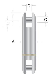
Electroline's Model SS-67 ocean-surface swivel is designed for above-water applications and features two clevis (fork/jaw) fittings with included pins. Constructed from stainless steel, the swivel has a grease-filled housing which is sealed to prevent water entry.
