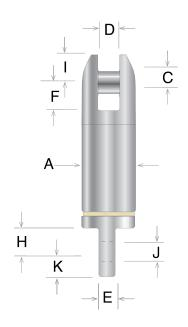
Electroline's Model SSP-68 industrial swivel is designed for sub-surface marine applications and features a clevis (fork/jaw) fitting with a pin and an eye-end fitting. Constructed from stainless steel, the oil-filled housing is sealed and pressure compensated to prevent water entry.
