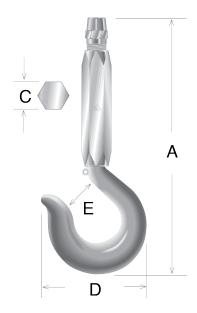
Electroline's non-swivel hook fitting features a swageless rope termination, allowing it to be quickly installed in the field without special tools or processes.
