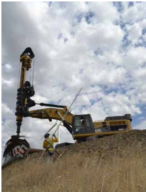
6000 Series Swivel - Directional Drilling - Dayton, WA
