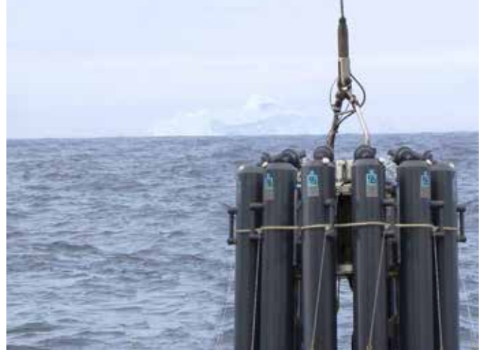
E-M Cable Fitting - Oceanographic Data Collection System - Antarctica
